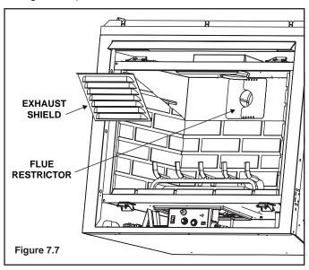
Break the Flue Restrictor into two pieces. Do this by bending the part back and forth until it breaks (see Figure 7.8).
